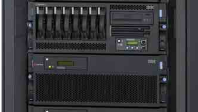
@server p5 550 rack system with I/O drawer
